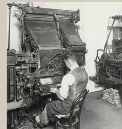
Linotype-Setzmaschinen, Kaufhaus Anthony Hordern & Sons, um 1935 © Public domain, Mitchell Library, State Library of New South Wales, Foto: AE Foster
