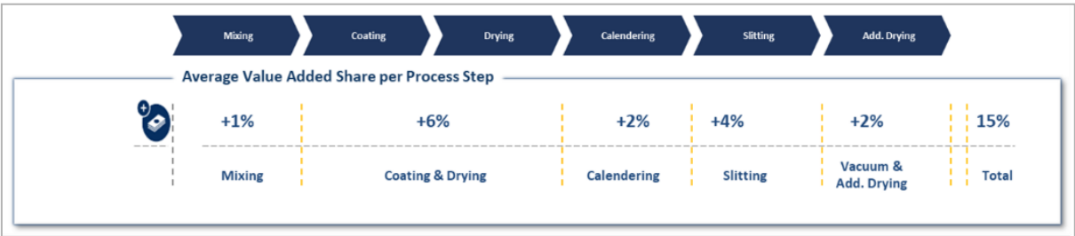
Figure 7: Overview of the electrode manufacturing process steps
